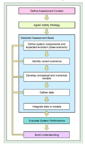
Safety assessment therefore involves: collating data; developing models both of components of the repository and its environment and the overall repository system; and performing safety analyses. In addition to numerical calculations, safety cases now include a broad range of evidence and arguments that complement and support the reliability of the quantitative analyses.
